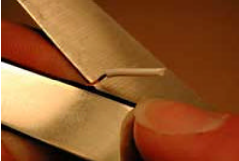
Strip insulation from the test lead.
