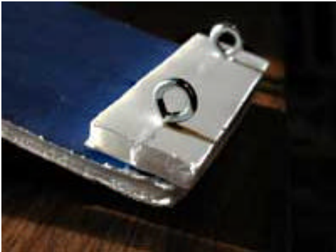
Turn the screw eyes firmly into the foam board.
