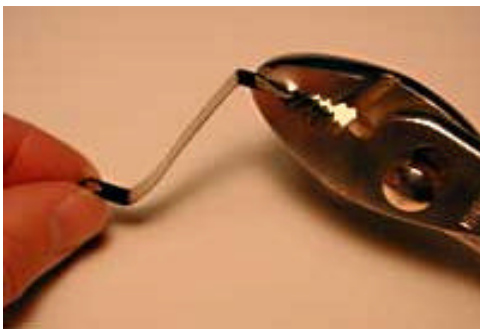
Use pliers to bend the metal connecting bar.
