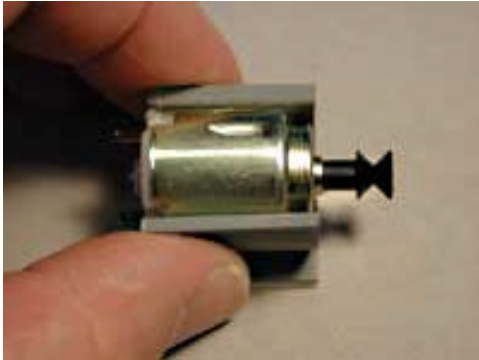
The electric motor in its mounting clip. .
