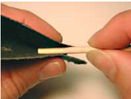
If necessary, sand the end of the axle to obtain a good fit with the wheel.
